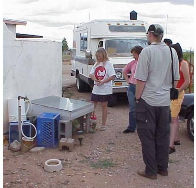
Fig. 3. Fall 2004 site visit to second generation solar distiller in use since 2001 with aluminum frame and water grade rated membrane at the home of July McClure in Columbus, New Mexico.
