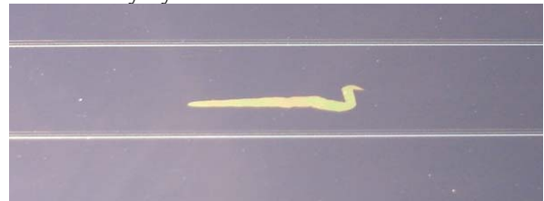
Fig. 4. Inconsequential manufacturing film scratch present on one of the Margaritas First Solar PV modules.
